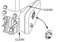
Muffler Area & Spark Arrester
