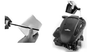
[2] Fill with fresh gasoline. Move throttle to FAST. (if equipped)
