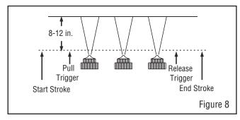
6. Overlap strokes just enough to obtain an even and fine coat on the workpiece. (See Figure 9)
