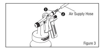
Set the operating air pressure to 30-50 PSI depending on the amount of fluid flow and atomization as required.
