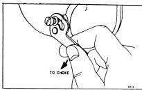
Move lever in direction of arrow to fully closed choke position. Set governor control in normal operating position.
