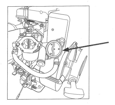
5. When the air cleaner base is reinstalled, tuck the fuel pump behind the base to prevent the outlet hose from interfering with the throttle lever.
