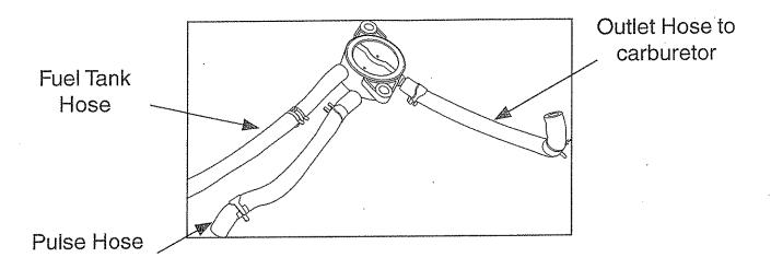
3. Connect the three hoses to the new fuel pump as shown above. Secure the hoses with hose clamps.
