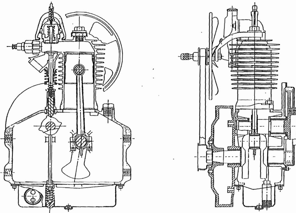
Cross Section of Type "P" Engine
