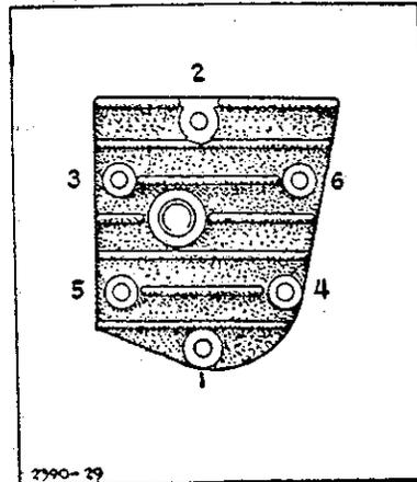
c. Use a socket wrench with a handle not over 6" long and tighten all screws evenly with a  $\frac{1}{4}$  turn in the rotation, 1 to 6, as shown in Plate No. 16. Do not tighten one screw down completely before the others as this may cause the cylinder head to warp or damage the gasket. Run engine two to five minutes.
