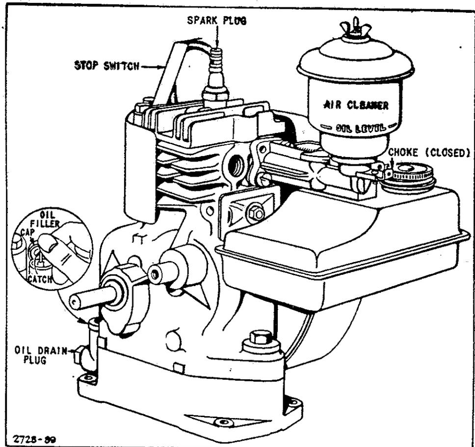
c. After the engine warms up, gradually open choke lever by pulling out until engine runs smoothly with the choke wide open. (A warm engine does not require as much choking as a cold one.)
