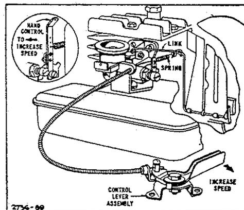
c. Place throttle in idling position. Engine should idle no slower than 1750 RPM, turn idle speed adjusting screw until this speed is reached.
