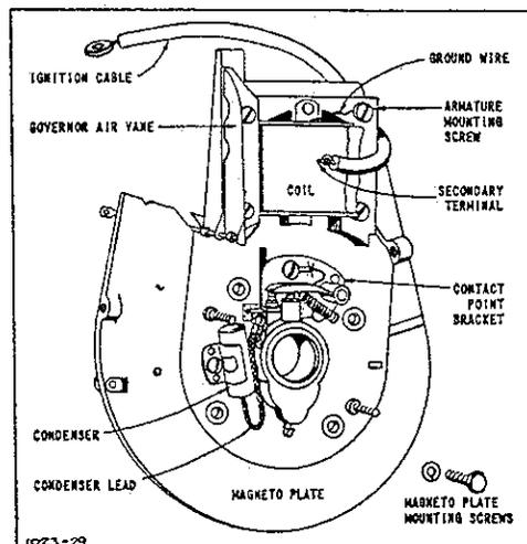
obtained tighten lock screw securely. If either or both points become badly pitted or burned, replace with complete new Contact Point Assembly, Part No. 29667.
