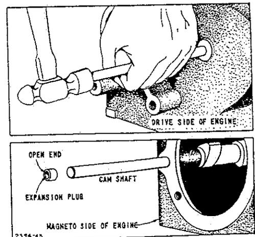
Be sure not to get burrs on the end of the shaft. After the shaft has been removed, check shaft for wear. If worn more than .001", replace with a new shaft.
