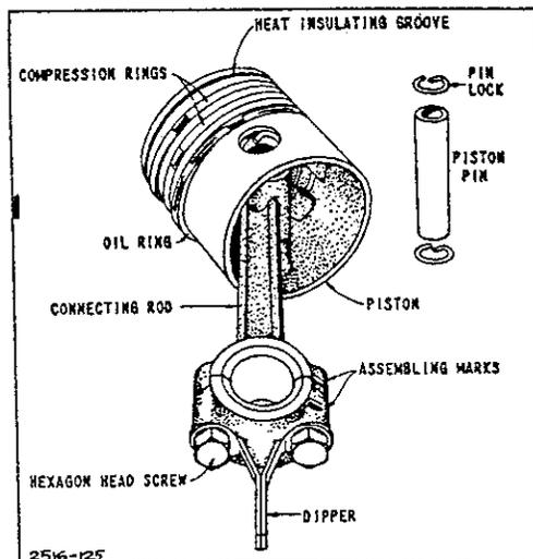
**49. PISTON RINGS.** The piston rings when fitted in the cylinder should have a gap of .007" to .017". The rings should be fitted in
