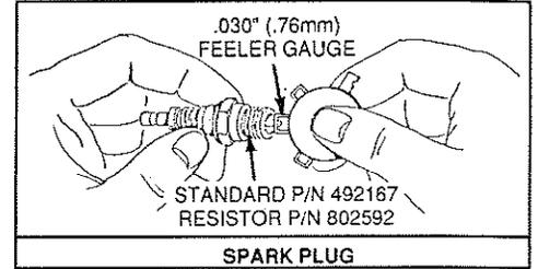
**NOTE:** Do not blast clean spark plug. Spark plug should be cleaned by scraping or wire brushing and washing with a commercial solvent.
