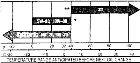
\* Air cooled engines run hotter than automotive engines. Use of multi-viscosity oils (10W-30, etc.) above 40° F (4° C) will result in high oil consumption and possible engine damage. Check oil level more frequently if using these types of oils.
