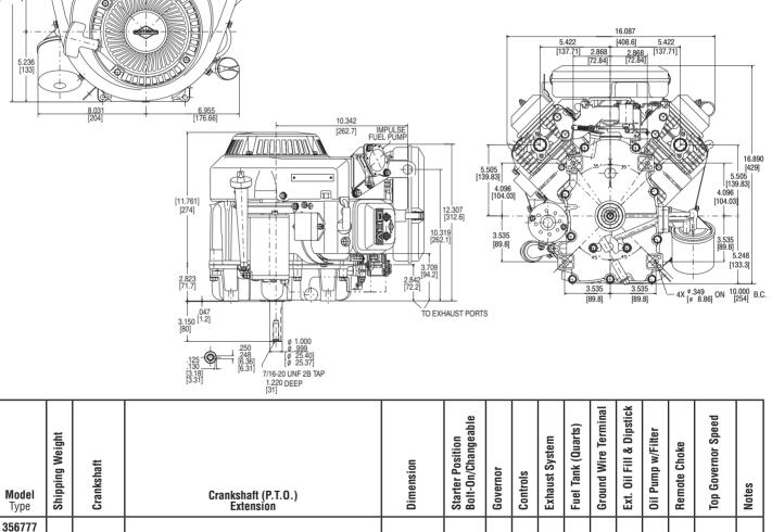
• Exhaust manifold and muffler omitted. See Briggs & Stratton Master Parts Catalog MS-4185 for Exhaust Manifold and Muffler Options.
