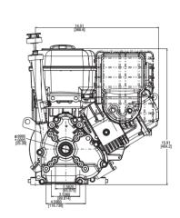
To make the center line of crankshaft the same as 190000 and 250000 Model Series, order 695154 spacer kit.
