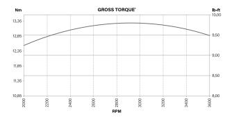
All torque levels are stated gross Nm per SAE J1940 as rated by Briggs & Stratton. "(Load @ 2'600 rpm). Fuel consumption is depending on engine configuration, application and operating conditions.
