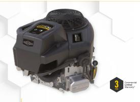
Engine type V-Twin, 4-stroke, air cooled, OHV (Overhead Valve) Model number 40T8 Series number Gross Torque (Nm) 39,57\* @ 3'600 rpm Displacement (cc) 656 Cvlinder Cast iron sleeve Bore & stroke (mm)  $75.4 \times 73.4$ Fuel tank capacity (I) NA Oil capacity (I) 1.9 Dry weight (kg) 38,1 **Dimensions** 497 x 462 x 399
