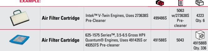
• The air filter cartridge in the normal Red Box Package is part number 499486S. It can also be ordered in the Display Parts Package under part number 5063. It can also be ordered in the Shop Pack Package under part number 4223 with a quantity of 6 filters in the box.
