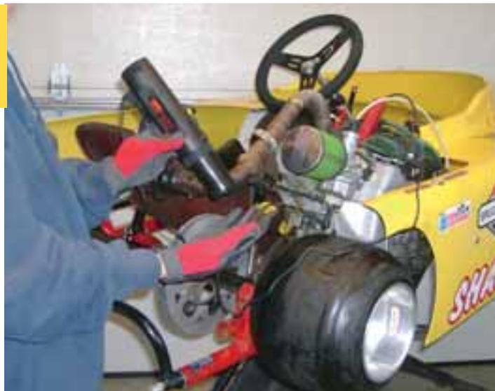
Always make sure to read the manufacturer's recommendations on the proper use of the timing light. Most importantly, don't be fooled by the fact that a timing light can make things like fans that are spinning 5,000 rpm, look perfectly still. Stay away from all moving parts when operating the timing light because looks can be deceiving.
