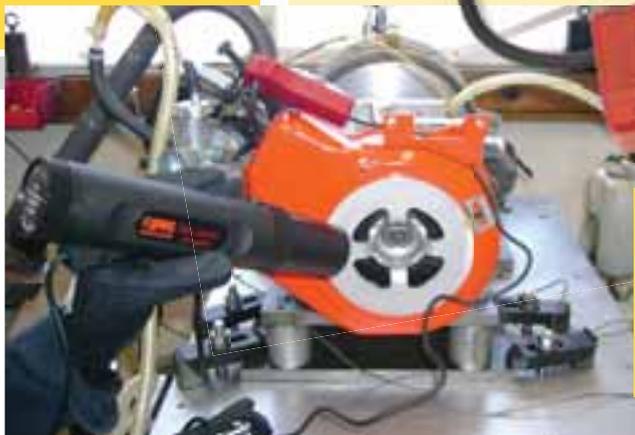
The primary use for a timing light is for setting the ignition timing. Though there are a couple ways to utilize it for checking the timing, the most common is a degree wheel and pointer fitted to the engine. When running the engine at a moderate speed the timing light will visually indicate where spark is occurring in reference to the crank angle.
