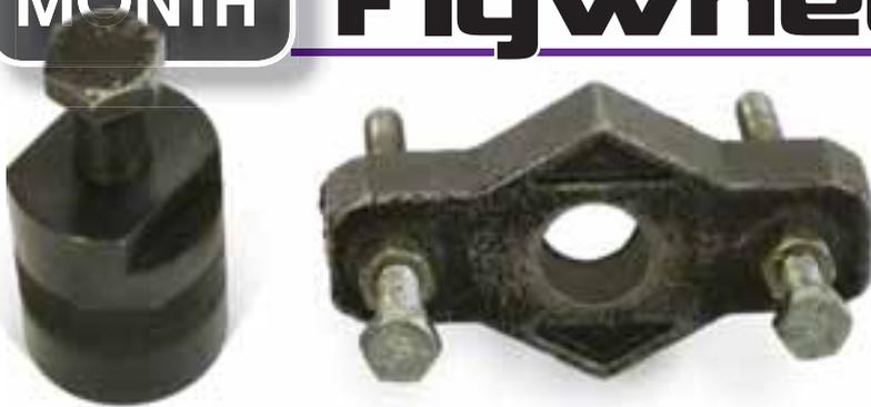
The new flywheel puller (left) can be seen here next to the older version. Both will work on the new PVL flywheel, but the new version is a more efficient tool for getting the job done. The new puller is specific to the racing engine and is made of high quality materials that will last through years of use by professional engine builders.
