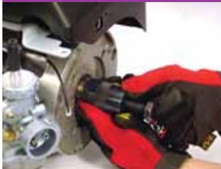
pullers for their racing engines: the older two bolt style that utilizes the fan mounting bolts on the Animal flywheel or the two specific puller holes on the World Formula's flywheel, and the new center pulling puller available for the new PVL flywheel. The older Animal flywheel puller can still be used on the new PVL flywheel; unfortunately the new PVL puller will not work on other flywheels.
