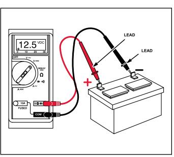
DC Voltage Battery Test
