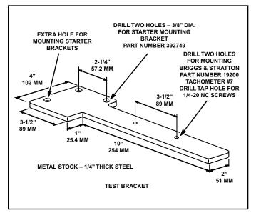
How to Make the Test Mounting Bracket
