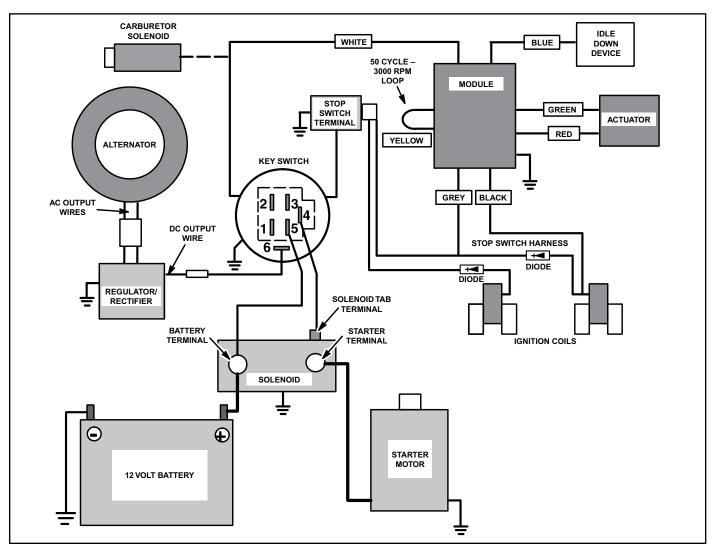
Performance Control Electronic Governor Wiring Diagram
