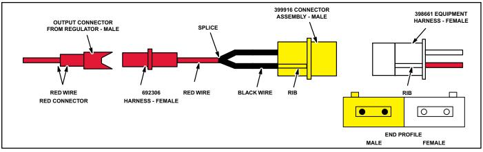
NOTE: THE DIODES MUST BE REMOVED FROM THE EQUIPMENT HARNESS.
