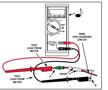
Tri-Circuit – Charging Circuit
