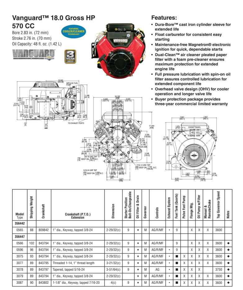
\* Oil fill and dipstick in cover; dual drain. See Briggs & Stratton Master Parts Catalog MS-4185 for Exhaust Manifold and Muffler Options.
