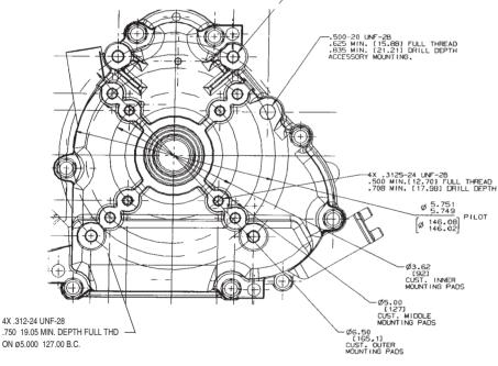
To make the center line of crankshaft the same as 190000 and 250000 Model Series, order 695154 spacer kit.
